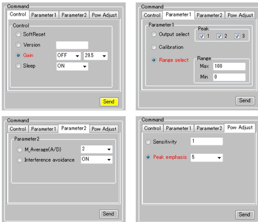
Command panel is used to send commands for MCU.
